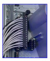
Series C field connections use a standard modular connector. The connector modularity allows for removal and insertion of the field wiring. This significantly reduces installation and maintenance procedures and can assist in field check out.
