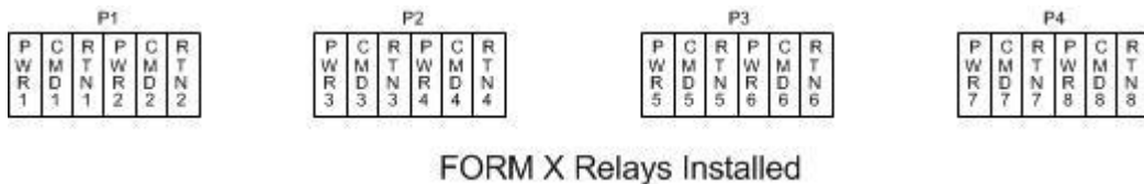
Figure 114: Terminal Block Connection for the Form X Relay Output with Contact Monitoring
