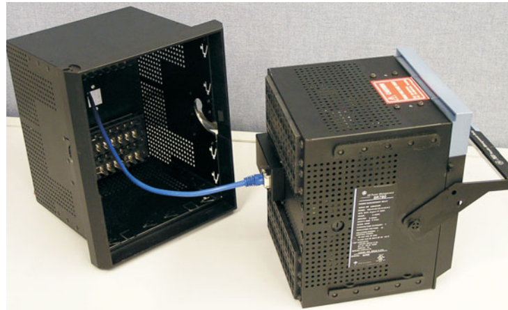
FIGURE 3-8: Ethernet Cable Connection
