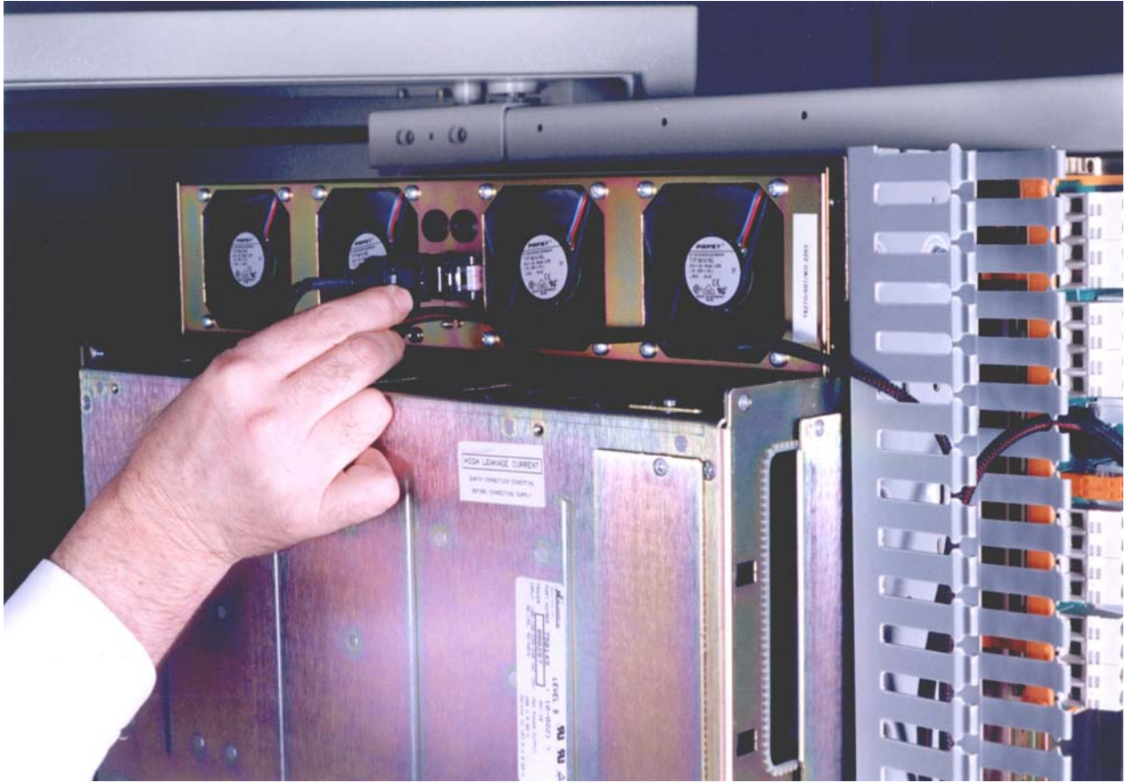
Figure 4-10: Connecting Power to a Fan Assembly
