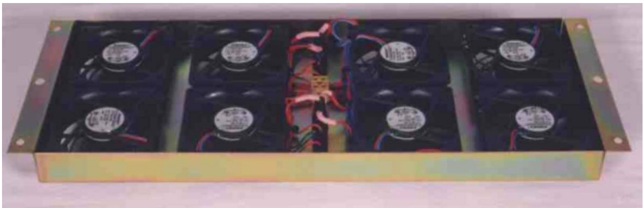
Figure 4-11: Roof Mounted Fan Tray
